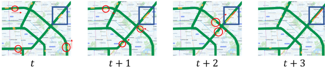
Fig. 1. An example of local traffic state propagation demonstrating the local spatial dependency in recent periods on Beijing [3]. The red circles indicate the traffic congestion on road locations and their moving direction, while the area inside the blue rectangle indicates the target location to be investigated.
